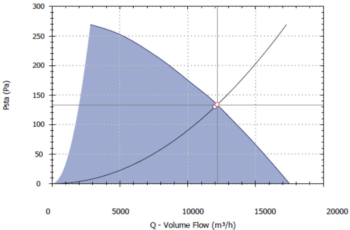
**Measurements, VN-Wall 714 T - 2.2 kW:**
