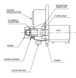
The mounting adaptor as well as specially shaped nut only for use with Model DB series Dials and Helicalohm pot. are fixed on the panel according to the illustration given left.
