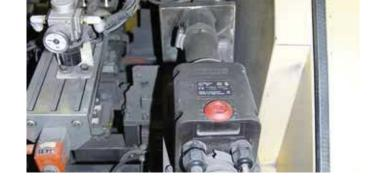
Deflashing foil sleeves from charcoal filter elements
