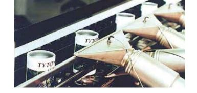
Utilizing precisely controlled hot-air to shrink PE sleeves on cans.
