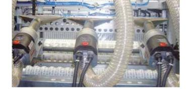
Three LHS 61S air heaters with wide slot nozzles in a wrapping line.
