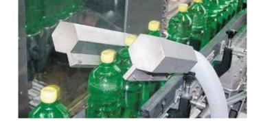
The combination of blow-off nozzles and blowers allows fast and efficient drying of beverage bottles.
