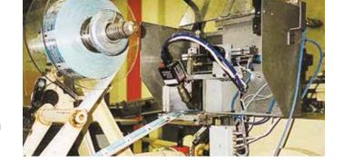
Air heater and blower for drying labels. Fast drying allows for high throughput speeds.
