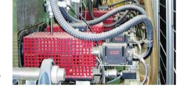
LHS air heaters in a production line for drying insulating material.
