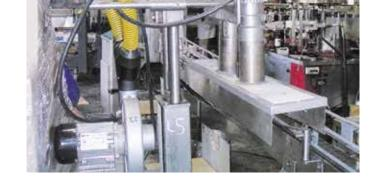
Two LE 10 000 HT air heaters and an ASO blower in combination with a shrink tunnel.
