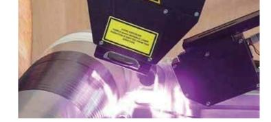
Welding of CFRP-Strips. (Image: MF-Tech, France, www.mftech.fr)
