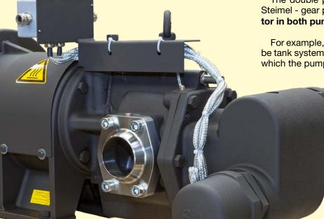
The double pressure relief valve of the SF / SFE 10 Steimel - gear pumps protects the pump and the motor in both pumping directions against overloading.
