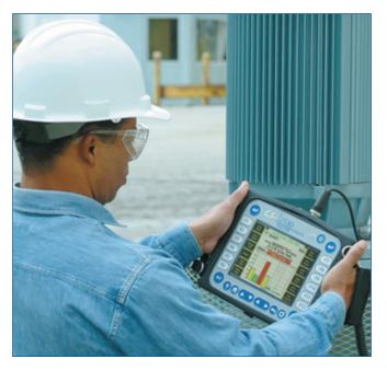
The Route application in the CSI 2130 uses pre-defined settings to provide instant feedback about machinery health in an easy-to-read color bar graph.
