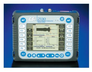
The Advanced Transient Analysis application records the vibration signature from machine startup, coastdown or during process disruptions for advanced analysis.
