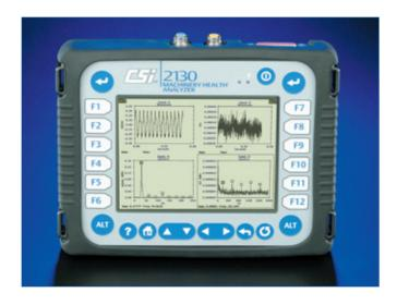
Fault frequency overlays is just one of many advanced analysis tools available in the field with the CSI 2130.
