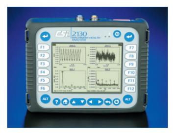
The full VGA screen displays standard and PeakVue data at the same time. The PeakVue plot (bottom right) provides clear indication of a rolling element bearing fault that is not visible in the standard reading (bottom left).
