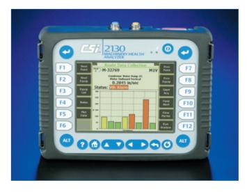
Complex data from vibration signals is condensed into machinery health information and presented in an easy-to-understand bar graph format. Details are available at the push of a button.
