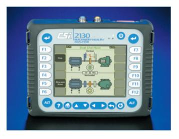
Applications for Advanced Balancing and Alignment make it possible to detect and correct machinery faults with the same CSI 2130.
