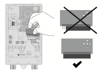
3. Push the antenna of the EnOcean® wireless module into the three housing openings of the control unit.
