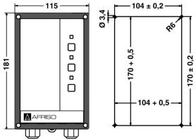
Fig. 7: Control unit with mounting frame for panel mounting; right: control panel cut out
