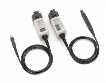
Differential active probes provide truer signal reproduction and fidelity for high-frequency measurements. With ultra-low input capacitance and versatile device-under-test connection capabilities, the TDP1500 and TDP3500 Differential-ended Active probes provide excellent high-speed electrical and mechanical performance required for today's digital system designs.
