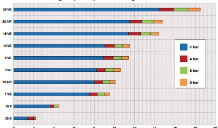
Dirt-holding capacity according to ISO 16889 (test dust: ISO-MTD) of different filter media and filtration grades. Dirt-holding capacities at 2, 4, 6, 8 bar pressure differential.
