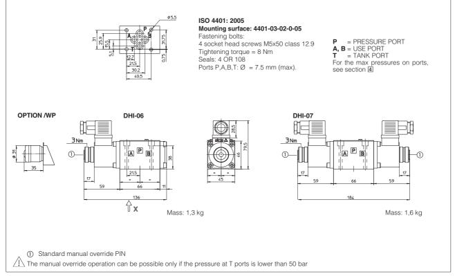
Overall dimensions refer to valves with connectors type 666
