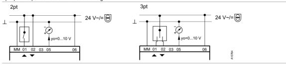
Modulating action with forced operation
