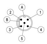
Fig. 8: M12 plug 5-pin+bridge
