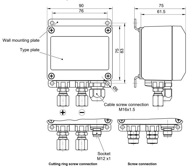
Fig. 10: Dimensional picture IP65 casing
