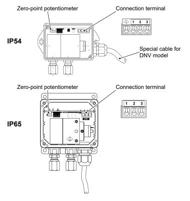
Fig. 7: Cable connection
