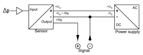
Fig. 6: 3-conductor circuit
