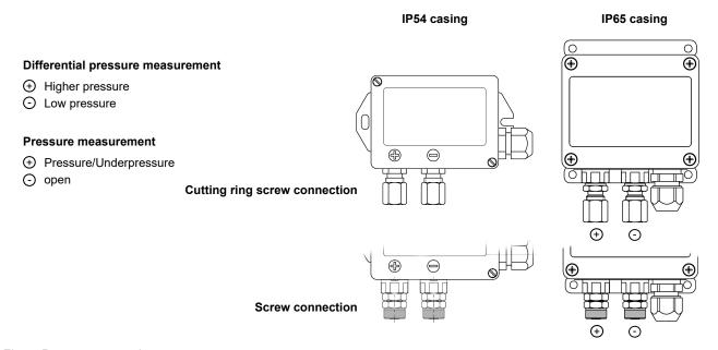
Fig. 5: Process connection
