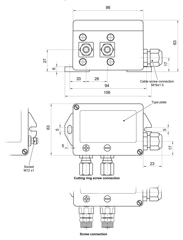
Fig. 9: Dimensional picture IP54 casing
