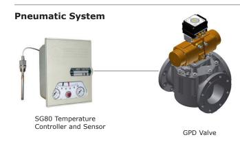
The pneumatic valve system incorporates a pneumatically actuated three-way control valve with controller and integral temperature sensor, the SG80, which can be panel or wall mounted. For more information on the SG80, see page 18. The pneumatic G valve system is ideal when there is a lack of electricity or when a fail-safe system is needed.
