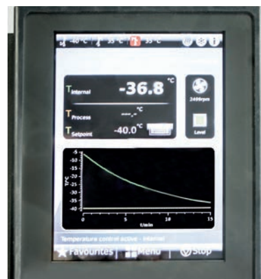
Sample temperature recording by optional immersion probe
