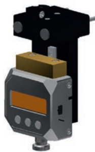
Shore 00 for parts testing / uneven surfaces
