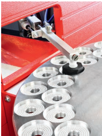
With direct tray-to-chamber handling, the sample arm picks samples from the tray. The testing area of 3000 Series is completely protected by a supervised safety door.
