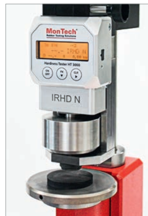
IRHD Normal measurement on parts
