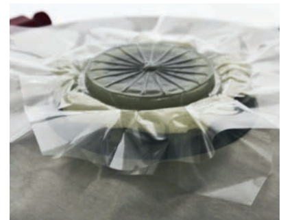
SBR Polymer sample after Mooney viscosity testing. Various types of testing film are available for easy sample handling, reduced cleaning needs, less die contamination and therefore improved repeatability.
