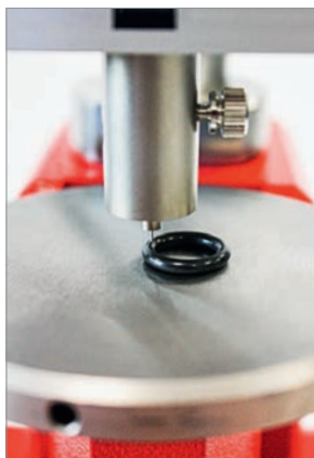
IRHD Micro measurement on O-Rings
