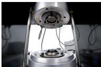
Die upgrades including precision heaters and probes
