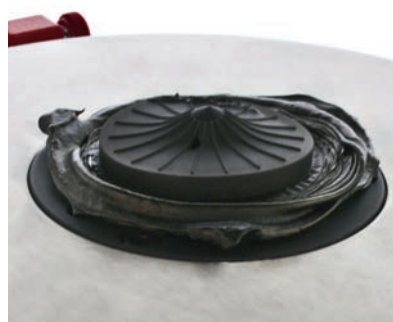
Rubber sample after Mooney scorch testing. Mooney Scorch testing is made simple with the V-MV 3000. Test can be automatically stopped once the maximum desired Scorch time or Scorch viscosity reading is reached, maximizing instrument availability and sample throughput.
