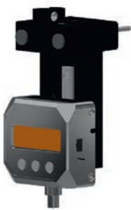
Shore M / AM for parts testing / uneven surfaces
