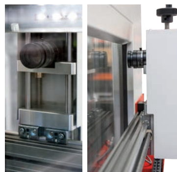
CCD Camera system for crack-growth measurement
