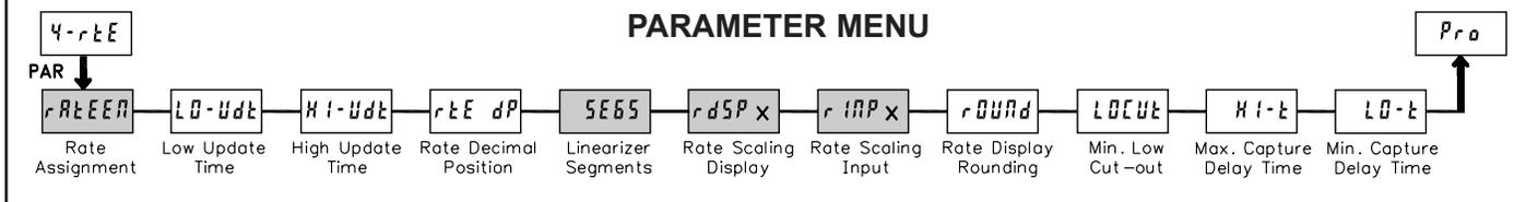
Module 4 is the programming for the Rate parameters. For maximum input frequency, Rate assignment should be set to **no** when not in use. When set to **no**, the remaining related parameters are not accessible. The Rate value is shown with an annunciator of 'r' in the Display Mode.
