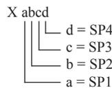
In Automatic Mode, the meter controls the setpoint output state. In Manual Mode, writing to this register (VX) will change the output state. Sending any character besides 0 or 1 in a field or if the corresponding output was not first in manual mode, the corresponding output value will not change. (It is not necessary to send least significant 0s.)
