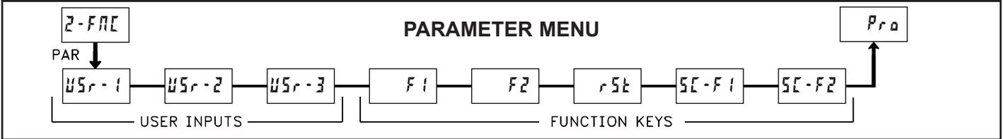
Module 2 is the programming for rear terminal user inputs and front panel function keys.
