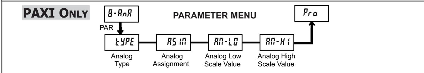
Module 8 is the programming for the analog output parameters. To have an analog output signal, an analog output plug-in card needs to be installed (See Ordering Information). For analog output hardware and wiring details, refer to the bulletin shipped with the plug-in card.
