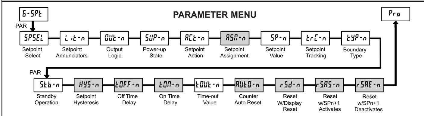
Module 6 is the programming for the setpoint (alarms) output parameters. To have setpoint outputs, a setpoint Plug-in card needs to be installed into the PAX (see Ordering Information). Depending on the card installed, there will be two or four setpoint outputs available. For setpoint hardware and wiring details, refer to the bulletin shipped with the plug-in card. For maximum input frequency, unused Setpoints should be configured for **OFF** action.
