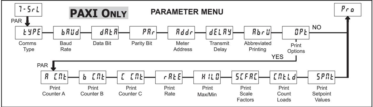
Module 7 is the programming module for the Serial Communications Parameters. These parameters are used to match the serial settings of the PAXI with those of the host computer or other serial device, such as a terminal or printer. This programming module can only be accessed if an RS232 or RS485 Serial Communications card is installed.
