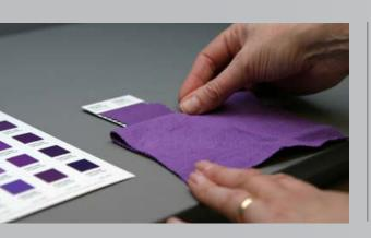
Colour requirements for manufacture and retail are complex and diverse. To ensure product colour, several types of light source are used (e.g. Artificial Daylight and a Point of Sale Light. Multiple light sources are also necessary to reveal colour inconsistencies and metamerism.
