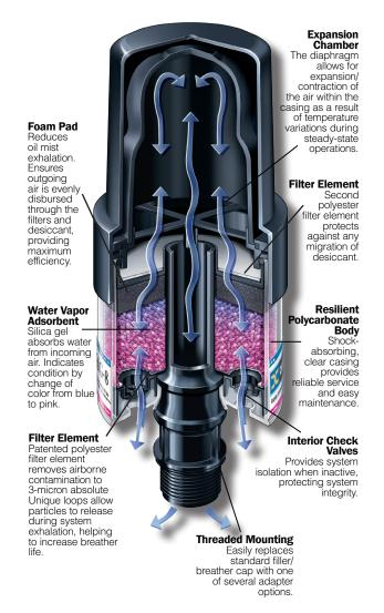
As wet, contaminated air is drawn through the unit, multiple 3-micron polyester filter elements remove solid particulate and the color-indicating silica gel extracts moisture.
