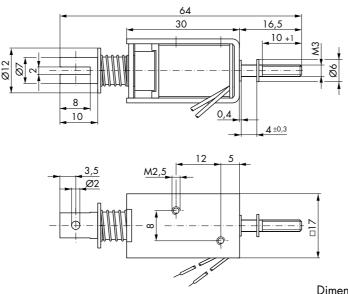
Dimensions given with armature in fully home position
