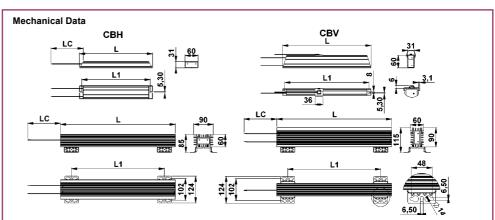
The external CLIP-ON thermo watch shown on CBV is also available for CBH. Internal thermo watch require 25 - 35 mm longer resistor profile, please require special data sheet.
