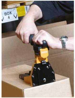
Fitted with a comfortable to use top grip and made from rugged aluminium, these manually operated tools are ideal for lower volumes of top sealing for single and double wall cartons.
