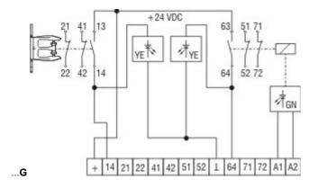
Protected against incorrect polarity and voltage spikes. limited terminating space 0,75 mm<sup>2</sup>
