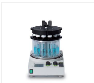
The Multivapor™ is a compact 6 or 12 position parallel vortex evaporator that is designed to optimize existing personal process workflows.
