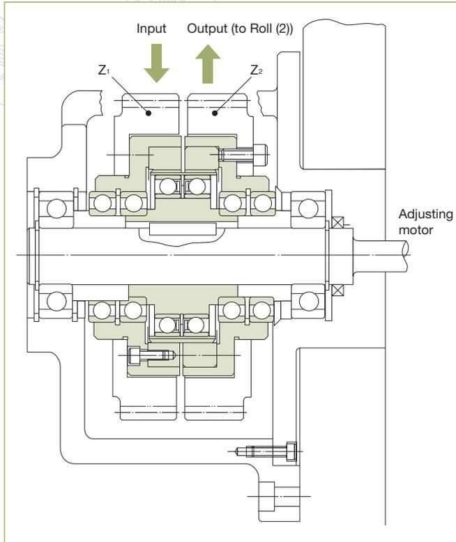
The figure is an example of a Harmonic differential gear unit (HDUA/FD-0) built in as a phase adjuster for the roll of a multicolor printer.
