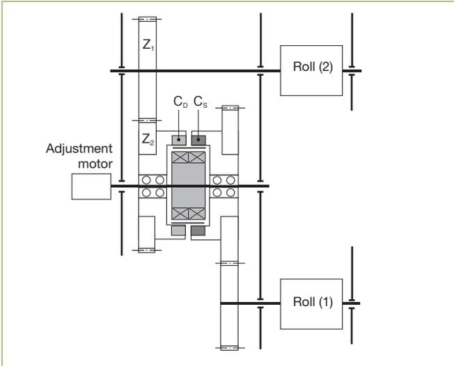
Brake a unit to adjust the phase of two rolls, normally an adjusting motor, and rotate it in the system: roll (1) → Cs → Cd → Roll (2). When the phase of Roll (2) against Roll (1) needs to be adjusted, the adjusting motor should be rotated. Stop the motor after adjustment and return Roll (2) to the original rotation.
