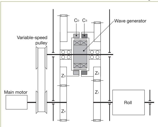
This is a unit to continuously make a slight change to the rotational speed of the roll. The rotation of the main motor has the following two routes.
