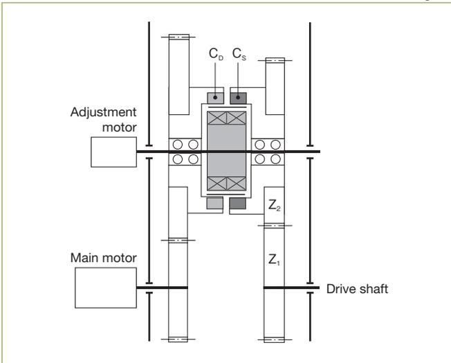
This is the method to fine-tune the speed and timing of the drive shaft by the adjusting motor without changing the rotational speed of the main motor.
