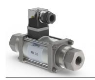
2/2 way valve direct acting pressure range PN 0-40 bar orifice DN 10 mm connection thread
