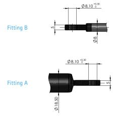
All dimensions in mm. The standard color of the tube and the piston rod is black.
