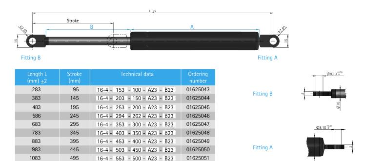
All dimensions in mm. The standard color of the tube and the piston rod is black.
