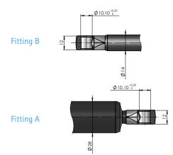
All dimensions in mm. The standard color of the gas spring and the piston rod is black.
