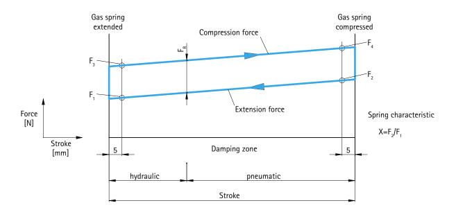
As seen in the graphic, the spring characteristic curve shows the force path of the gas spring over the stroke, from the extended to the retracted state and back. The spring characteristic illustrates the balance of power of  $F_2/F_1$ . For the design of gas springs, the force  $F_1$  is, in addition to the dimensions, the most important criterion.
