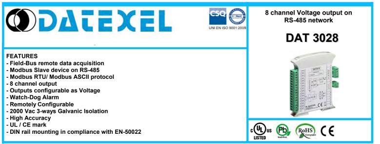
GENERAL DESCRIPTION The DAT 3028 device generates 8 output analog signals from digital commands. The data are transmitted with MODBUS RTU/MODBUS ASCII protocol on the RS-485 network (RS-232 interface is available). It is possible to generate voltage signals up to 10V.
