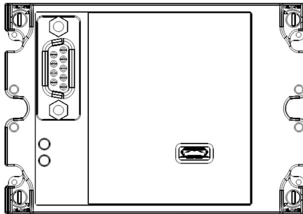
Connection to the Profibus module using USB micro type B (Modbus RTU) and RS485 DB9 (Profibus DP-V0).
