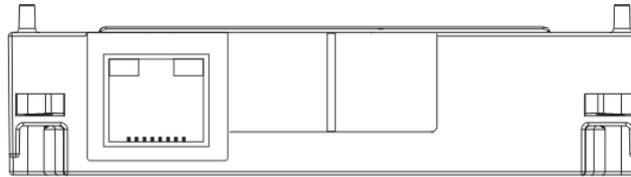
Connection to Ethernet or BACnet modules using the RJ45 connector.
