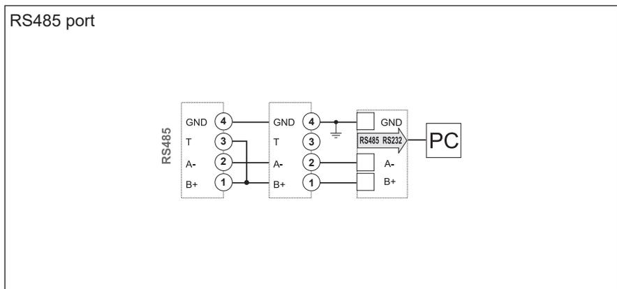
**NOTE.** RS485: additional devices provided with RS485 are connected in parallel. The termination of the serial output is carried out only on the last instrument of the network, by means of a jumper between (B+) and (T).
