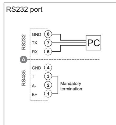
**NOTE.** RS485: additional devices provided with RS485 are connected in parallel. The termination of the serial output is carried out only on the last instrument of the network, by means of a jumper between (B+) and (T). The **A** communication RS232 and RS485 ports **can't be** connected and used simultaneously.
