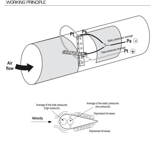
Section in plane blade limiting head losses (<3%) and turmoils.
