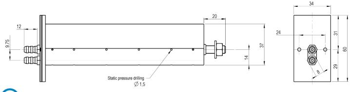
Total and static pressure ports location according to the LOG-TCHEBYCHEV\*\* method.
