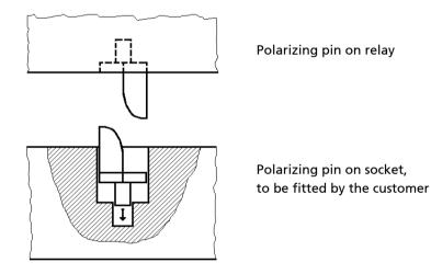
Whilst the use of this component is optional, it is nonetheless strongly recommended where there are multiple relays installed on an electrical panel, for example:
