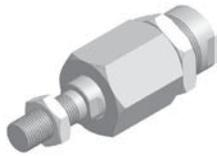
Flexo coupling for articulated mounting of piston rod. Flexo fitting is intended to take up axial angle errors within a range of  $\pm 4^\circ$ .
