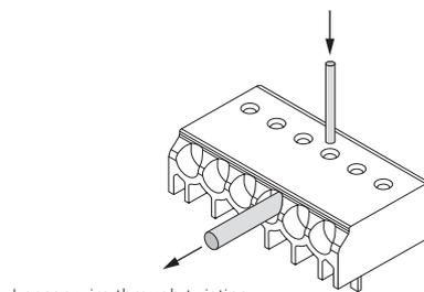
Loosen wire through twisting and pulling or using a Ø 1 mm release tool
