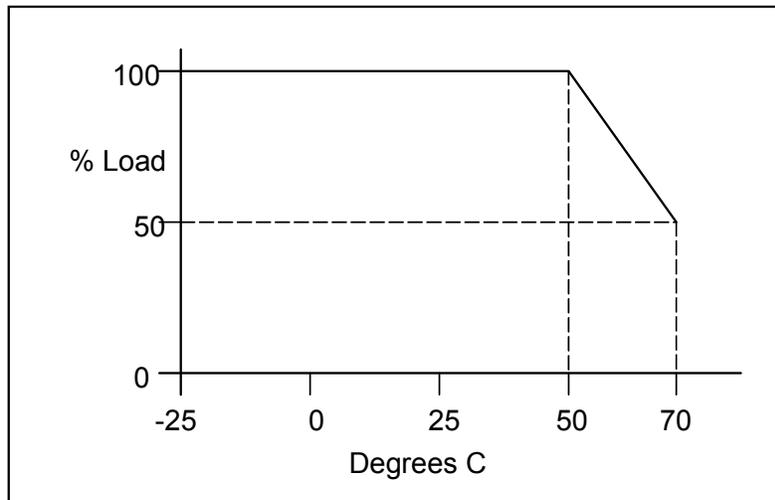
**Figure 3-1 XL125 Output Power vs. Ambient Temperature Envelope**
